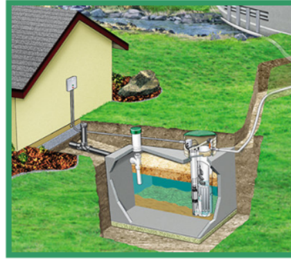
STEP TANK EFFLUENT PUMPING SYSTEM
